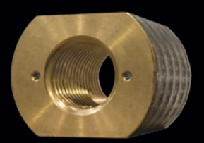
With a guaranteed self-locking, heavy steel lifting screw and a premium alloy bronze load nut, it is undoubtedly the ultimate in safety. The self-locking ACME threaded screw has been a constant in our long history, spanning more than 40 years. It is guaranteed failsafe, environmentally friendly, having no hydraulic oil to leak, and has a proven lifetime of 15 years or more.
