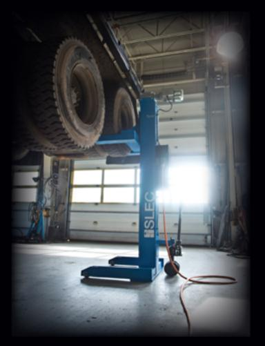
The detachable remote can be connected to any column. This is more convenient than being limited to a single column, and is much safer, because it places the operator exactly where they need to be.
