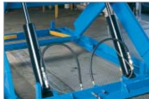
Rod side of each cylinder is vented to the hydraulic reservoir to eliminate contamination
