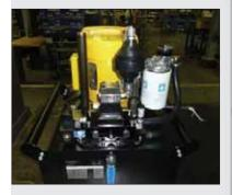
A ZW-series pump, including an unloading circuit, designed to power four separate load stations in a machining center.
