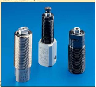
Threaded cylinders for workpiece positioning, holding and ejecting applications where space is at a premium. The advance and retract mode of double-acting models allow installation of clamping accessories to the plunger for pull and push action. Cylinders can be mounted with horizontal bracket to position the workpiece against the stops. Ideal for supporting or positioning a part.
