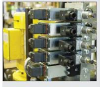
Five Enerpac VP-series solenoid valves mounted to a ZW-series electric pump provide complex circuit control in a compact package.
