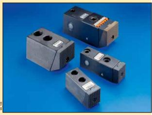
Enerpac pull down clamps are designed to allow unobstructed top face machining. Independent horizontal and vertical movement achieves high lateral and pull down forces to hold the workpiece firmly down against the machine table or fixture. The pull down forces are approximately 33% of the clamping force.
