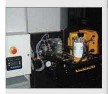
A custom PLC with push button controls and power unit to operate an Enerpac automatic coupler system.
