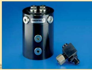
Rotary couplers are specially designed unions to transfer pressurized fluid from a stationary supply line to a rotating device. Used for workholding or clamping device such as fixtures installed on rotating index tables.
