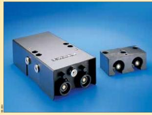
The automatic coupler system allows connection and disconnection of palletized hydraulic circuits. This system eliminates the direct intervention of an operator, allowing hands free, safe functioning of the process. Typical systems include one base station located at the load/unload station operating one or more pallet receivers.
