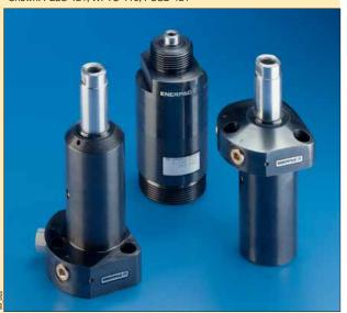
Hydraulic pull cylinders utilize hydraulic pressure to hold down parts in a fixture. The guided plunger maintains orientation during the full clamping cycle, eliminating the need for an external guide. Internally threaded plunger ends accept various custom attachments to assist in the clamping process.
