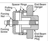
1748 **End Bushing Adapter Puller Set for Hendrickson Truck Suspensions**
