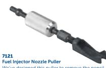
We've designed this puller to remove the pencil-type fuel injector nozzles used in many agricultural and construction engines. The slide hammer action gives a straight, even pull without damaging components.
