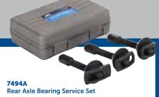
Designed to make the removal of semi-floating rear axle bearings easier. Allows you to capture the bearing firmly, distributing the pulling force over the entire bearing. This reduces damage and increases the amount of applications. Set includes three pullers to service most domestic cars. Use with OTC Nos. 1155 or 1156 slide hammer with 5/8"-18 UNF thread. Pullers also available separately.
