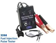
Fuel injector testing requires precision equipment. This vehicle powered tool fills that requirement. It enables you to check cylinder balance by firing individual injectors at 1/2-second increments in three different ranges: 1 pulse of 500 milliseconds, 50 pulses of 10 milliseconds, 100 pulses of 5
