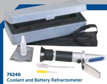
This can be used for measuring the freezing point of either propylene and ethylene glycol based cooling systems. It can also be used for checking the strength of electrolyte solution in batteries. This precision instrument features high quality optics with ultra smooth focusing on the body. Coolant scale range:  $32^{\circ}$  F/0° C to  $-60^{\circ}$  F/  $-51^{\circ}$  C. 75234
