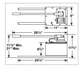
Pump and valving mount on common cover plate; permits use on other than standard OTC reservoirs.
