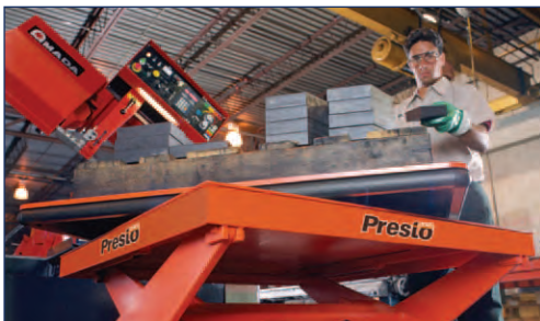
Standard Turntable shown mounted on Hydraulic Lift
