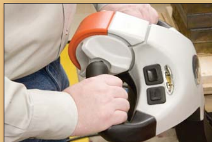
Auto reversing "belly bump" switch protects against operator accidents while working in tight quarters
