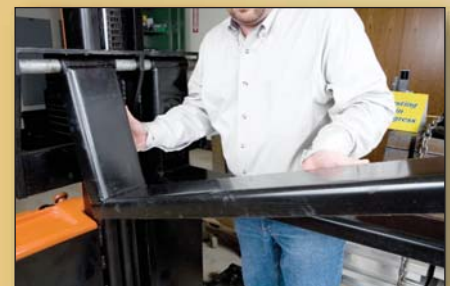
Adjustable fork carriage allows forks to be quickly repositioned to best accommodate loads (straddle only)
