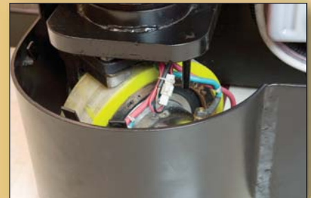
Smooth polyurethane drive wheel is fully shrouded to protect operators' feet
