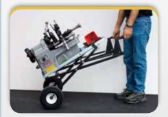
7090 mounted on 60508 collapsible cart.
