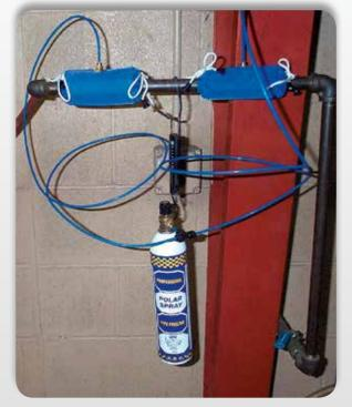
Wheeler's Pipe Freeze Kits install in seconds on pipes up to  $2^{3}/_{8}$ " O.D. and require no special tools. Ice plugs last 15–20 minutes and can be easily renewed.
